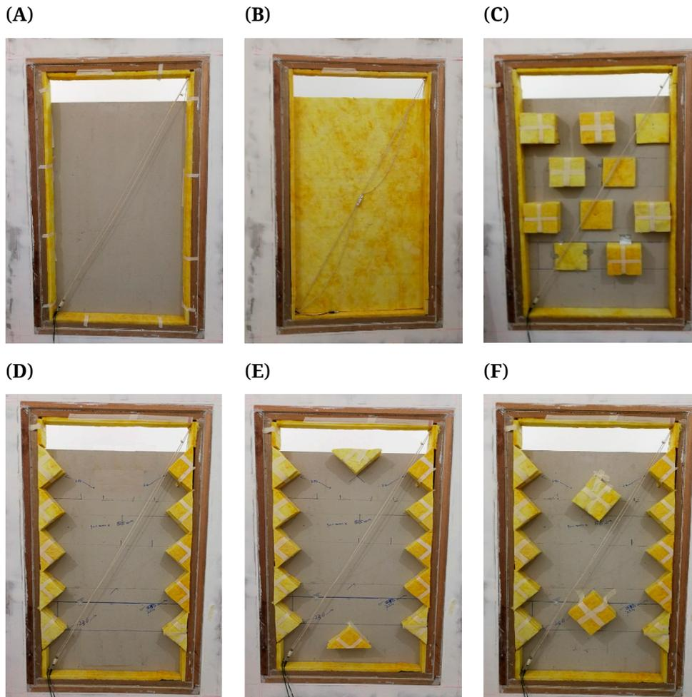
**Figure 4.** Six ventilation partitions with acoustical treatments. (A) Case C1, STC 22; (B) Case C2, STC 31; (C) Case C3, STC 32; (D) Case C4, STC 26; (E) Case C5, STC 29; (F) Case C6, STC 32.
