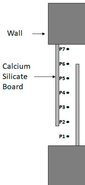
**Figure 3.** The cross-section view of Case B0: Ventilation partition without any acoustical treatment.
