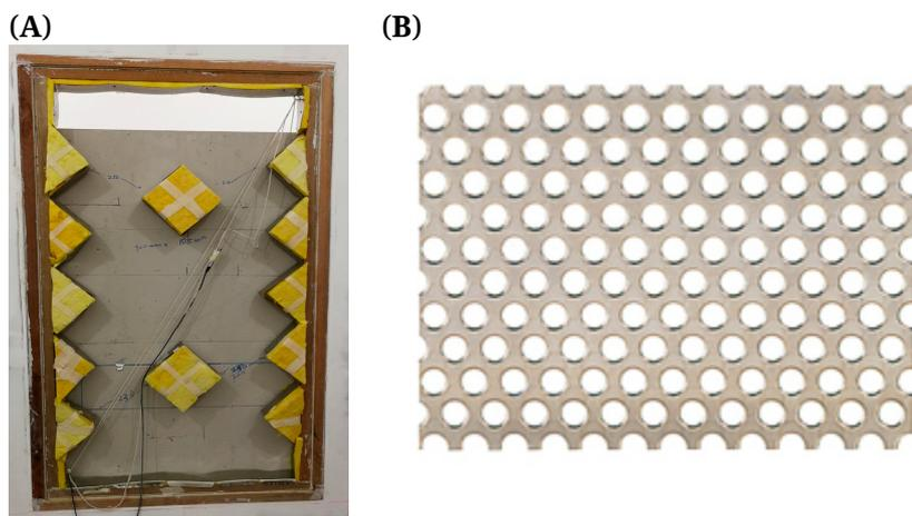
Figure 6. (A) Case 6-1: with perforated metal sheet, STC 30. (B) Perforated metal sheet.
