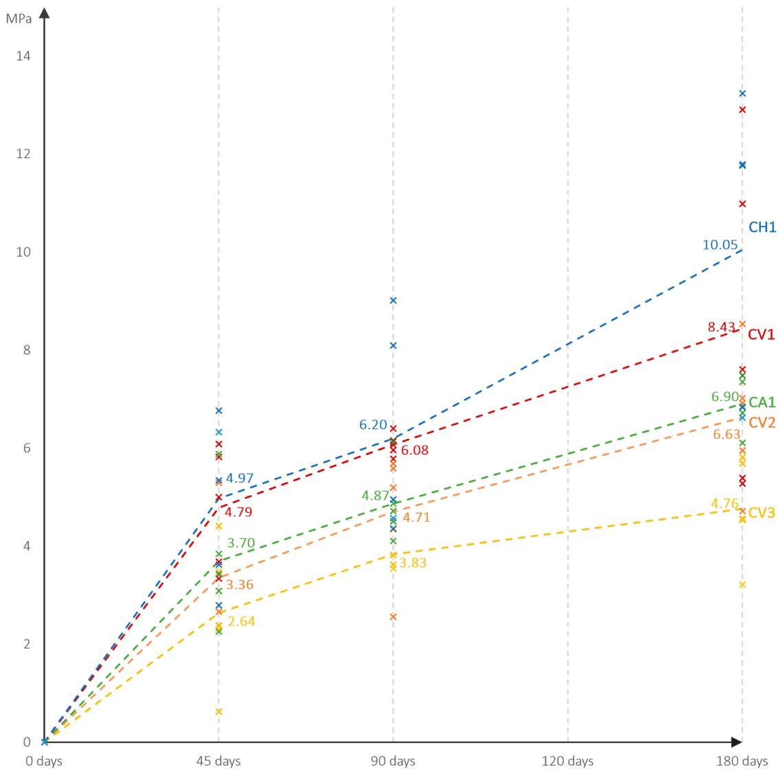
**Figure 10.** Evolution of mean compressive strength of test samples over time, showing the MPa values of each test sample type at 45, 90 and 180 days.
