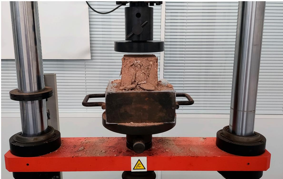
**Figure 8.** Compression tests using a hydraulic press at the Department of Architectural Constructions at Universitat Politècnica de Valencia.
