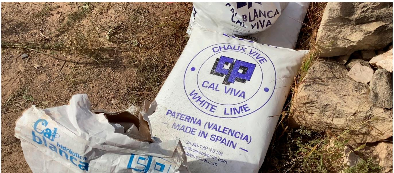
**Figure 2.** Types of earth and lime used in the research: stone and powdered quicklime, hydraulic lime NHL-3.5 and powdered hydrated air lime.
