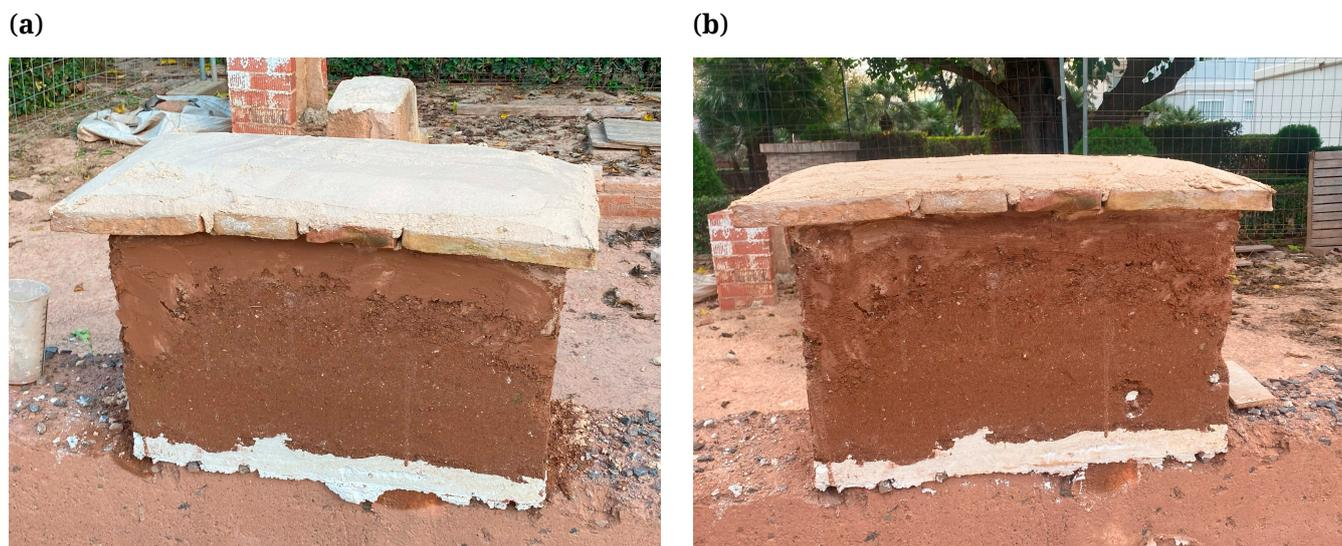
**Figure 9.** Appearance of a superficial calcrete or bulge on wall T1. **(a)** Wall surface on the day of the execution. **(b)** Wall surface the day after execution, showing a calcrete of considerable size.
