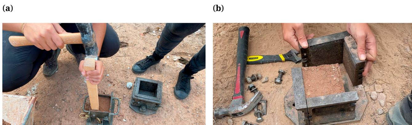
**Figure 7.** Execution process of test samples. (a) Filling and compacting moulds. (b) Process for dismantling moulds after a prudential amount of time.
